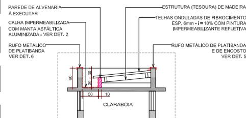
**DET. 4 - DETALHE GENÉRICO CORTE TELHADO CLARABÓIAS - A EXECUTAR 1:25**
