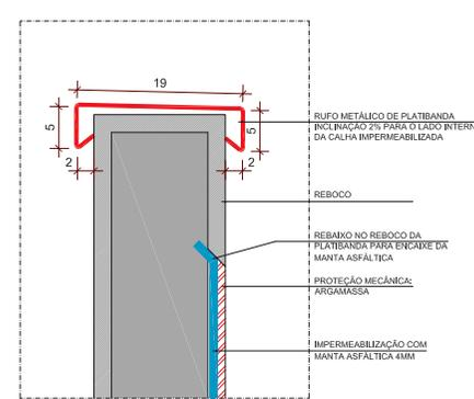
**DET. 6 - DETALHE GENÉRICO RUFU METÁLICO DE PLATIBANDA 1:2**
